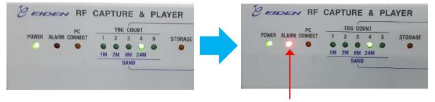
The light of the ALARM indication LED is detected.
